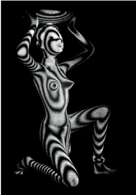
Fig. 2.19. Two-wavelength contour fringes
